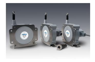
The SG1 provides absolute linear position up to a 10-ft. stroke range. Constructed with a rugged polycarbonate body, this model is available in an 80-inch or 120-inch stroke range and offers optional IP67 protection for wet or outdoor installations and an M12 connector for easy installation.
